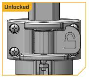
Lock Collar is locked and the Shaft is secure; when the Unlock from is visible, the Stow Lock Collar is unlocked and will not hold the Shaft in place. When locking or unlocking, be sure to press the Lock Arm so that it is fully seated against the Stow Lock Collar.
