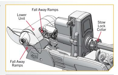
NOTICE: To secure the motor in place and prevent accidental deployment when stowed, lock the Stow Lock Collar (a). Be sure to press the Lock Arm so that it is fully seated against the Stow Lock Collar.
