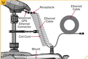
To install the Ethernet Cable, align the pins on the Advanced GPS Ethernet Connector with the Receptacle on the Ethernet Cable. Notice the keyed connectors. Tighten the Collar from the Ethernet Cable to secure the connection.
