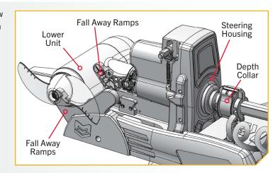
**NOTICE:** To secure the motor in place and prevent accidental deployment when stowed, slide the Depth Collar down against the top of the Steering Housing and close the Cam Lever to lock the Depth Collar.
