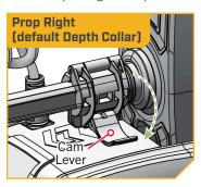
If the Stow Orientation is changed to Prop Right, the Depth Collar must be rotated on the shaft to improve accessibility. The Depth Collar is positioned correctly on the Shaft when the Cam Lever opens upward when the motor is stowed.
