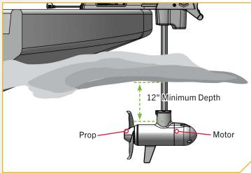
**NOTICE:** Ensure that the top of the lower unit is submerged at least 12" below the surface of the water to avoid churning or agitation of surface water.
