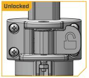
Lock Collar is locked and the Shaft is secure; when the Unlock from is visible, the Stow Lock Collar is unlocked and will not hold the Shaft in place. When locking or unlocking, be sure to press the Lock Arm so that it is fully seated against the Stow Lock Collar.
