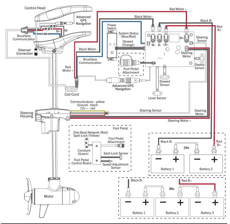
**NOTICE:** This is a multi-voltage diagram. Double-check your motor's voltage for proper connections. Over-Current Protection Devices are not shown in this illustration.
