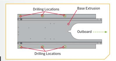
**NOTICE:** The mounting surface for the Riptide Terrova QUEST must be flat. Rubber Washers can be used to shim the Base Extrusion flat before hardware is tightened.
