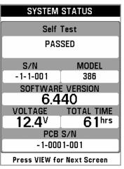
**Self Test** displays results from the internal diagnostic self test, including unit serial number, Printed Circuit Board (PCB) serial number, software revision, total hours of operation, and the input voltage.
