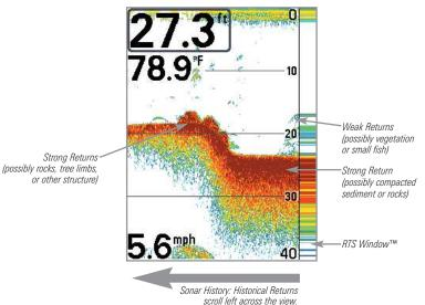
Use **Bottom View** to select the method used to represent bottom and structure on the display. See *Sonar Menu Tab* to set the Bottom View.
