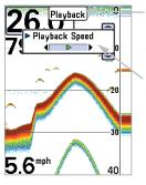
"Playback" indicates the control head is playing a saved recording.
