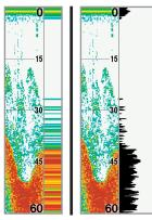
The Wide RTS Window™ indicates the sonar intensity through the use of a bar graph. The length of the plotted return indicates whether the return is weak or strong. The depth of the sonar return is indicated by the vertical placement of the return on the display depth scale. The Wide RTS Window<sup>™</sup> does not use grayscale.
