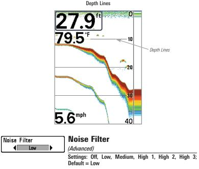
**Noise Filter** adjusts the sonar Noise Filter to limit interference on the display from sources such as your boat engine, turbulence, or other sonar devices.
