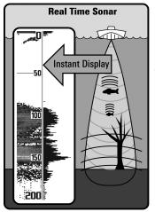
SONAR is an acronym for SOund and NAvigation Ranging. Sonar uses precision sound pulses or "pings" which are emitted into the water in a teardrop-shaped beam.
