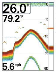
**<u>Structure ID</u>**<sup>®</sup> represents weak returns in blue and strong returns in red when Sonar Colors is set to Original. If the Sonar Colors palette is changed, the Structure ID<sup>®</sup> will display the strongest return as specified by the palette. See *Sonar Menu Tab: Sonar Colors* for more information.
