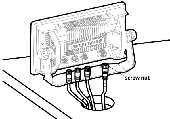
6. Connect each cable to the appropriate ports on the control head. The ports are labeled, and the connectors are keyed to prevent incorrect installation.
